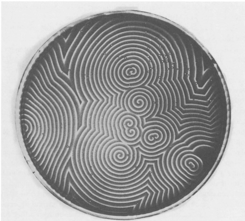
Fig. 5.7. Chemical waves observed in the Belousov–Zhabotinsky reaction in an unstirred medium (Winfree, 1972a).
